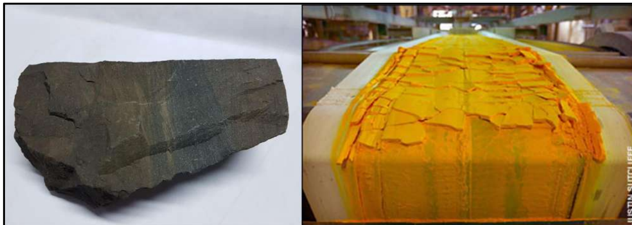
Figure 1-2: An example of sandstone uranium ore and the final uranium oxide product (yellowcake)
